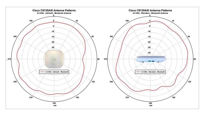
**Figure 2.** Antenna profiles
