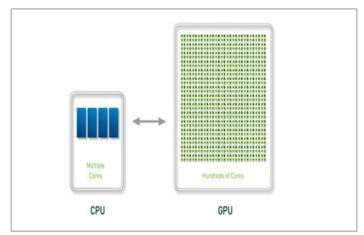
Fig.1: Core comparison between CPU and GPU [1]
