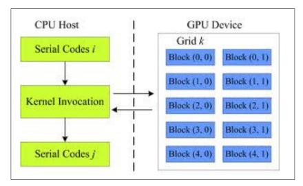
Fig.2: Flow of execution of GPU [2]
