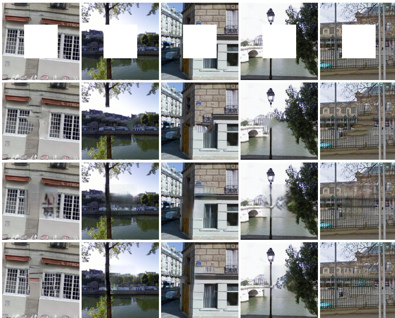
Figure 10. Visual comparisons of Paris Streetview result. From top to bottom: input image, Content-Aware Fill, Context Encoder ( \ell_2 and adversarial loss) and our result. All images are scaled from 512 \times 512 to fit the page size.
