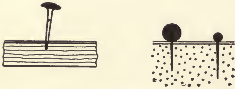
Fig. 186. A Contrast Between Long, Cloth-covered Map Tacks which are Likely to Fall Out, and Glass-head Map Pins Made with Short Needle-points so that the Pins May be Pushed in until the Heads Touch the Map
