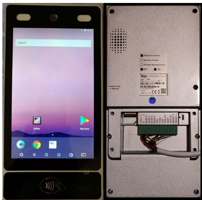
Figure 10. The front and back of the Telpo access control device
