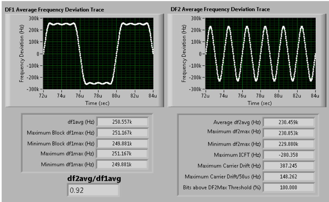
**Figure 31. Modulation Characteristic Measurement on Low Energy Bluetooth signal (LabVIEW)**
