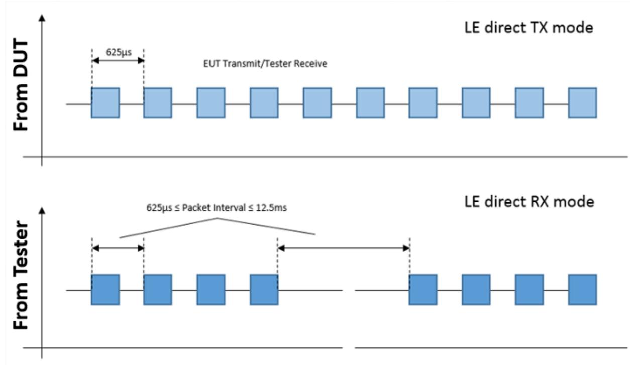
Figure 22. Direct Test Mode Packet Timing
