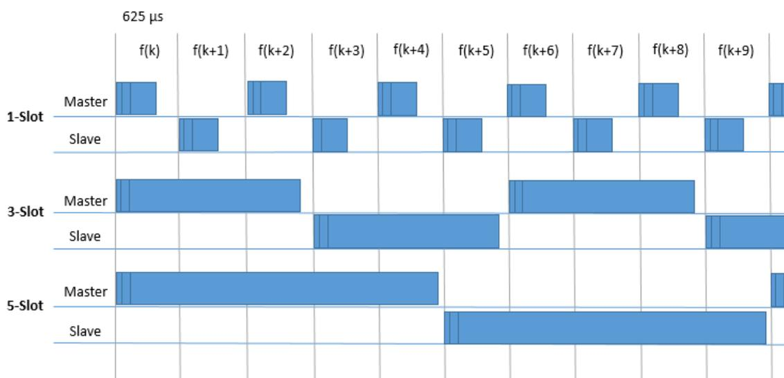
Figure 14 Packet Slot and Timing Structure
