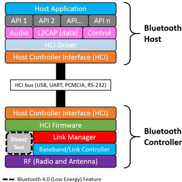
**Figure 2 Bluetooth System Stack**
