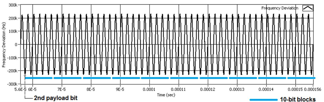
Figure 36 CFO Payload Deviation Trace (100us of the 37-byte LE payload containing 10101010 pattern)
