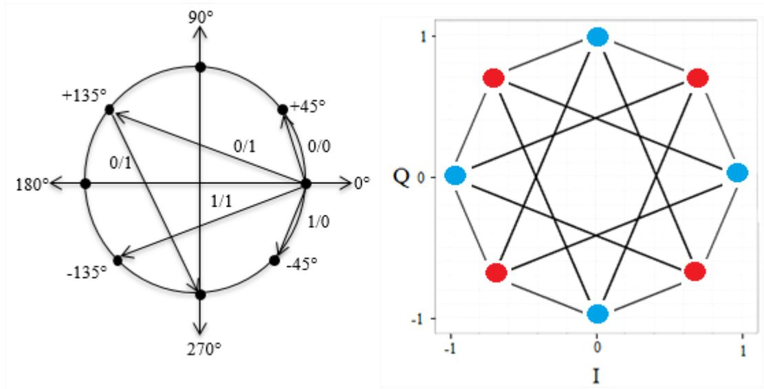
Figure 9  $\pi/4$ -DQPSK Symbol Map and Constellation Plot
