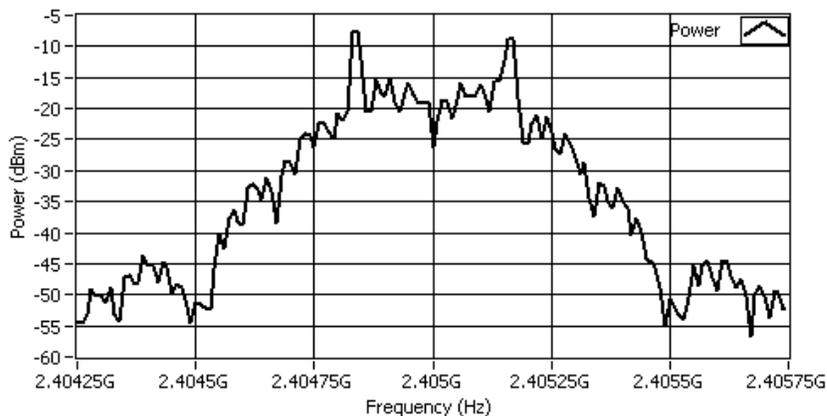
**Figure 8 Frequency Representation of the GFSK Modulated Signal (HV1 burst with 10 bytes payload, 10 averages)**
