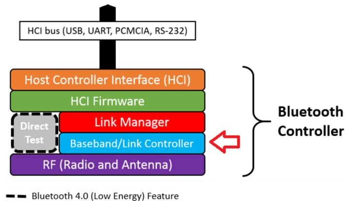
Figure 11 Location of Baseband Physical Layer in Bluetooth Protocol Stack
