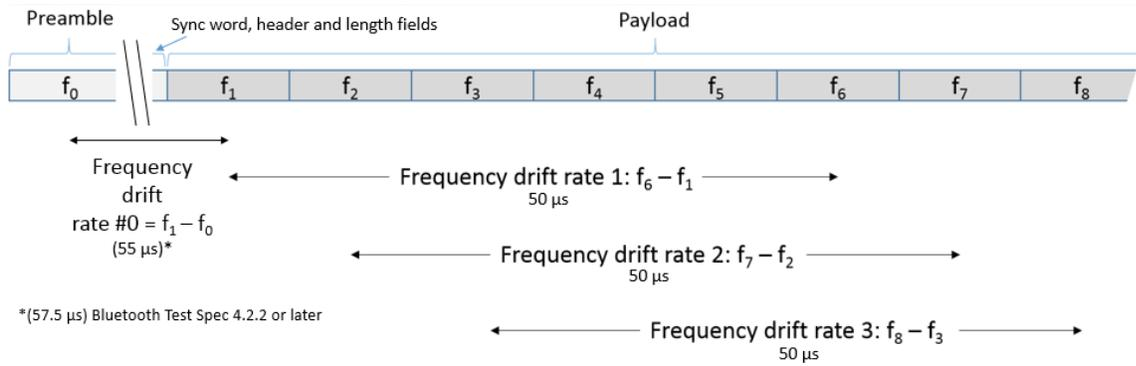
**Figure 37. Frequency drift rate measurement principle**
