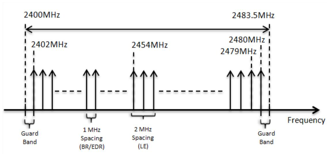
Figure 5. Bluetooth Frequency Bands and RF Channels
