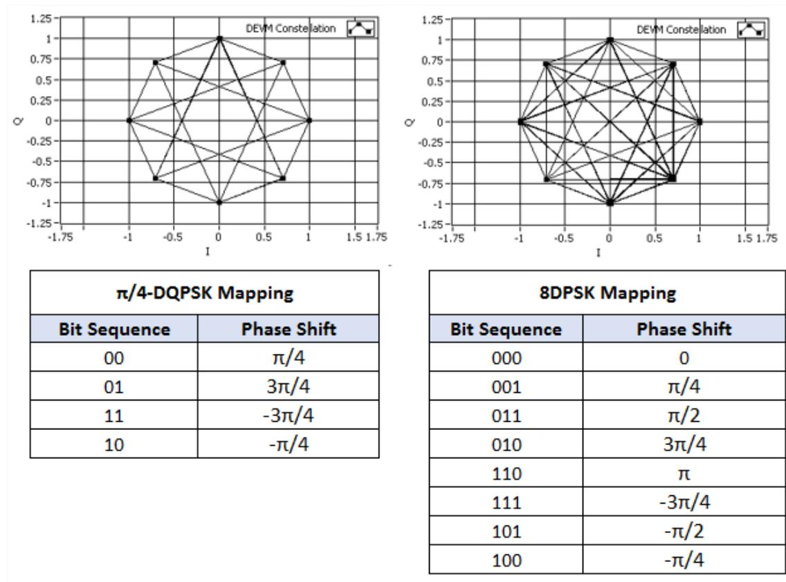
Figure 40. Bits to Constellation Symbols Mapping
