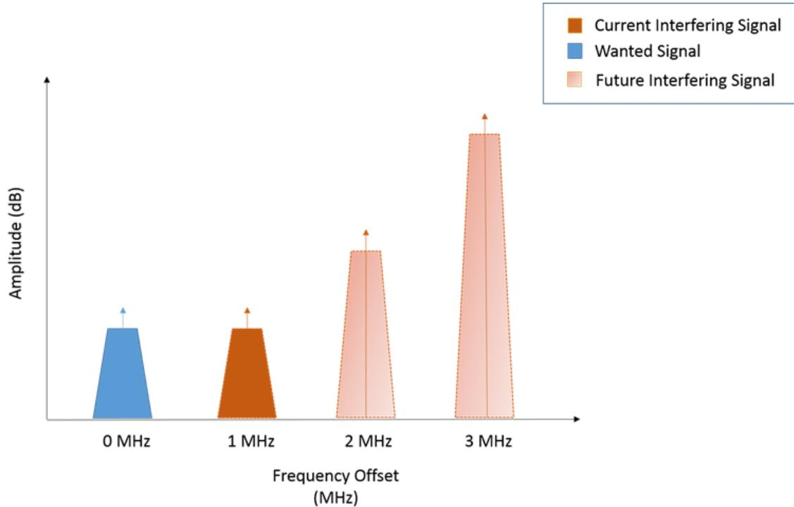
**Figure 52. Relationship of Interfering Signal to Wanted Signal (Image is not to scale)**
