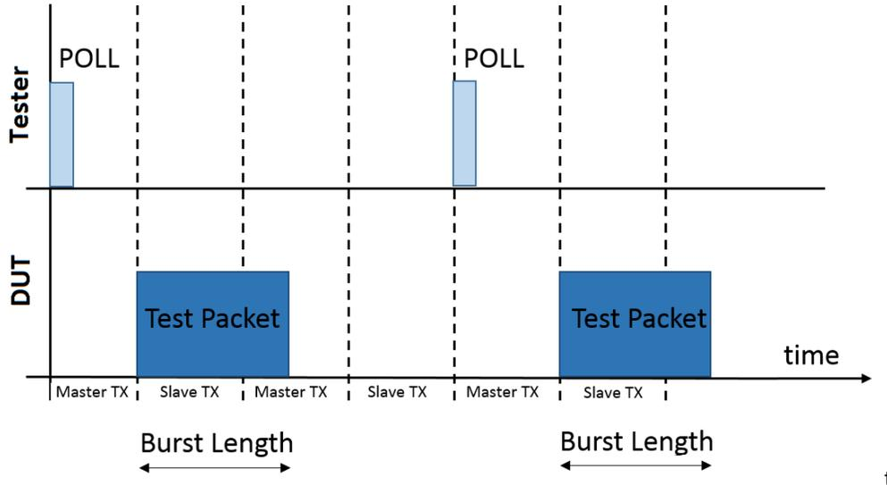
Figure 19. Transmitter Test Timing
