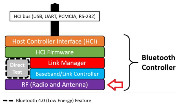
Figure 4. Location of RF Physical Layer in Bluetooth Protocol Stack
