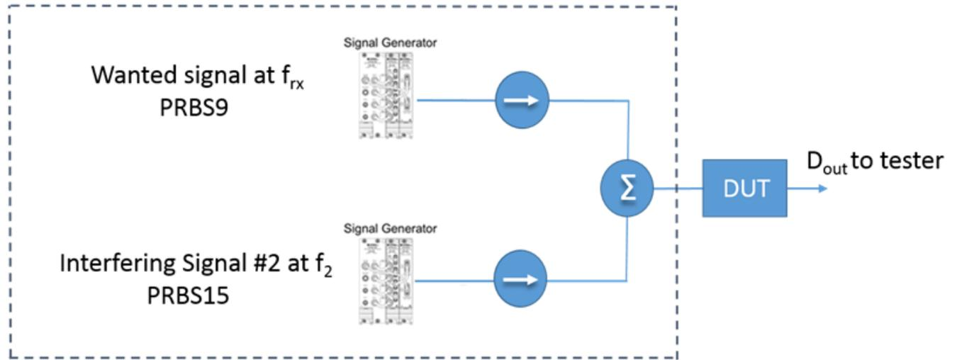
Figure 51. Hardware diagram for C/I test
