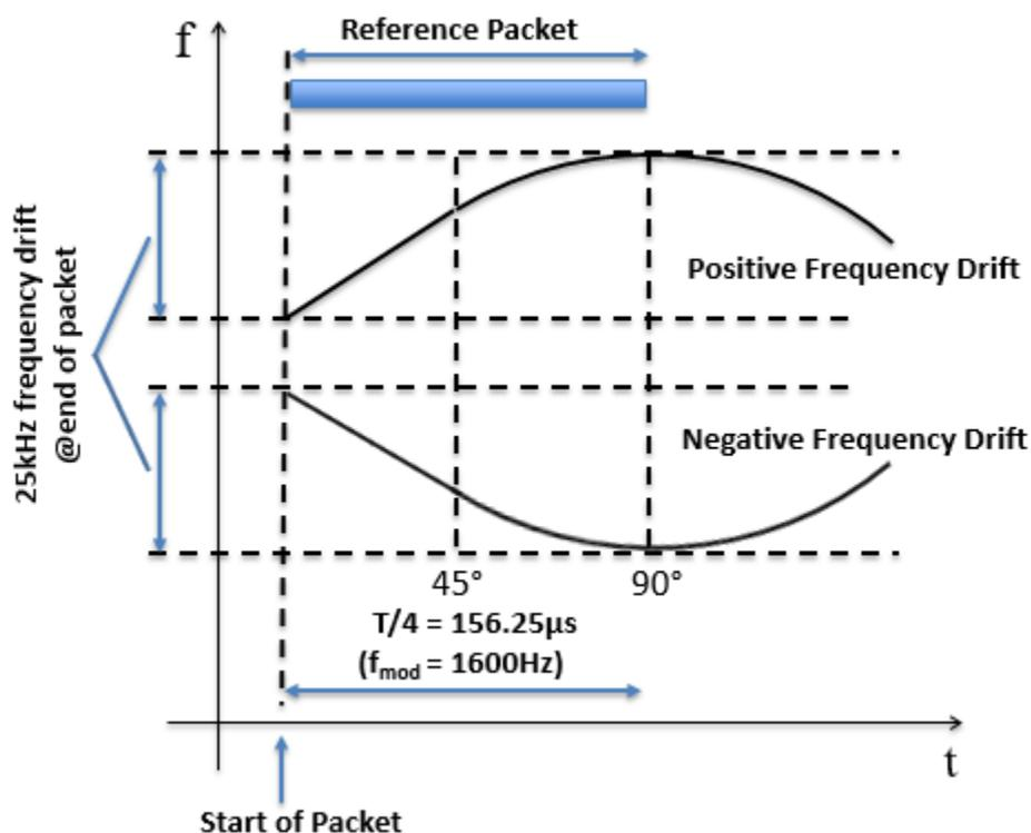
Figure 47 Dirty Transmitter Frequency Drift Emulation Principle (BR, single slot)
