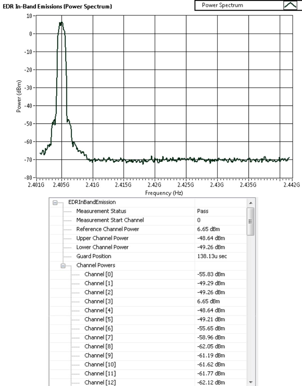
Figure 45. EDR In-band Emissions (40 channels shown)
