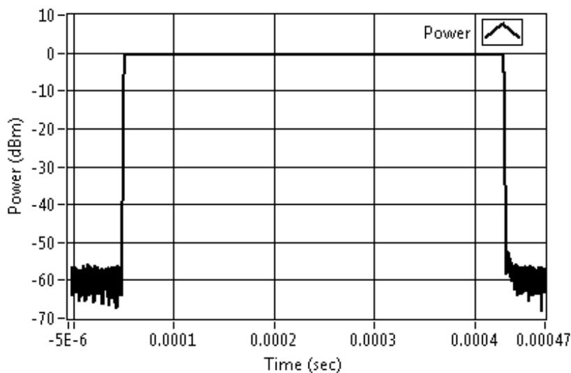
**Figure 7. Time Representation of GFSK Modulated Signal (HV1 burst with 10 bytes payload at 0dBm)**
