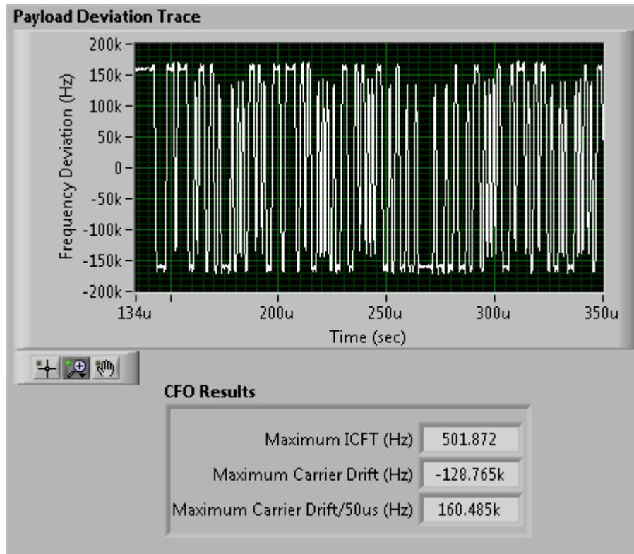
Figure 33. ICFT measurement on a DH1 packet with full payload (216 bits) at 2.405GHz (10 averages)
