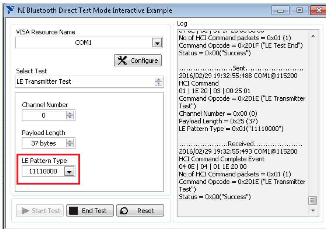
Figure 23. Generation of LE packets with 11110000 payload pattern using the Bluetooth DTM Interactive Panel
