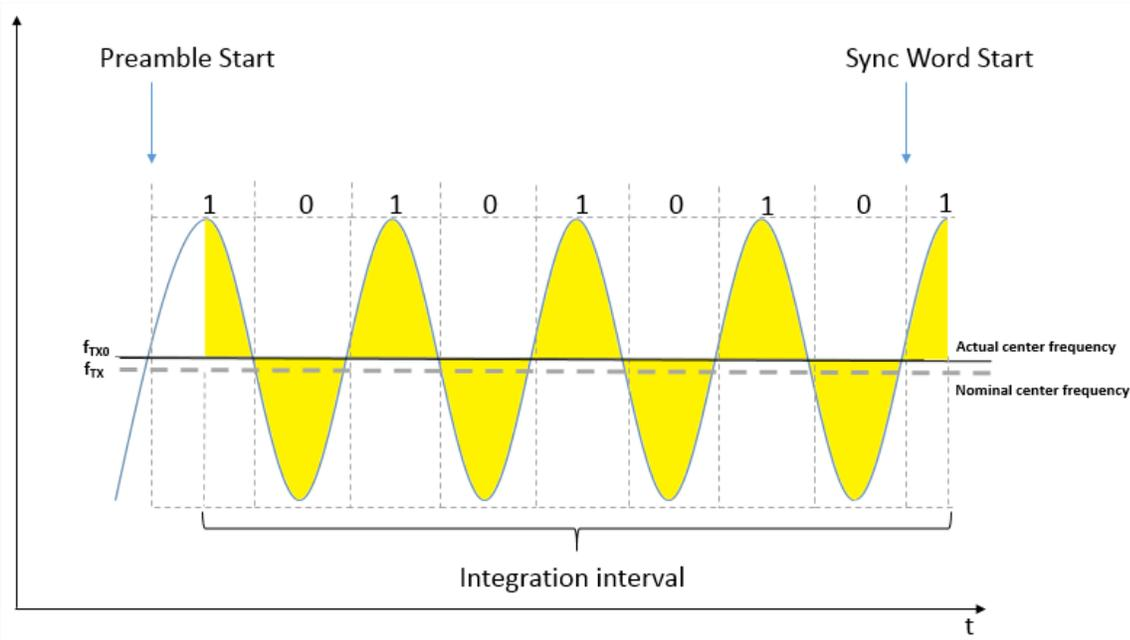
Figure 34. Initial frequency offset ( $f_0$ ) measurement principle (Low Energy Packet)
