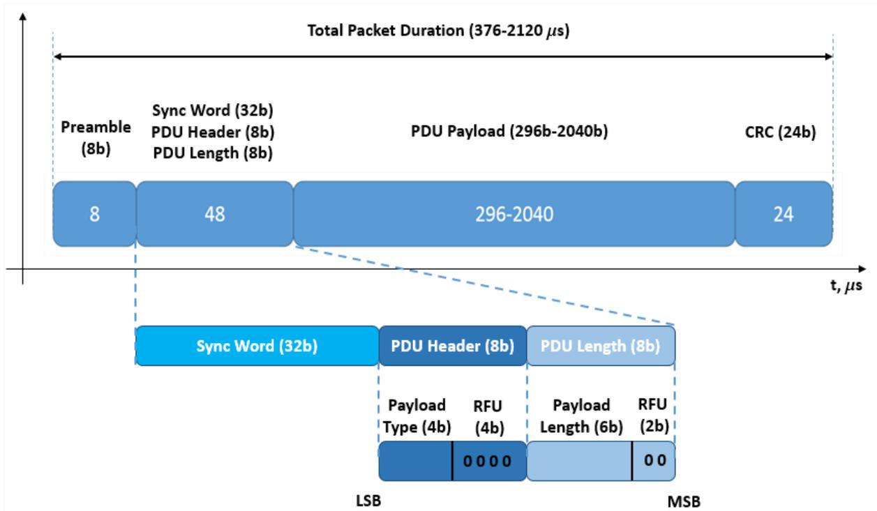
Figure 21. BTLE Direct Test Mode Packet
