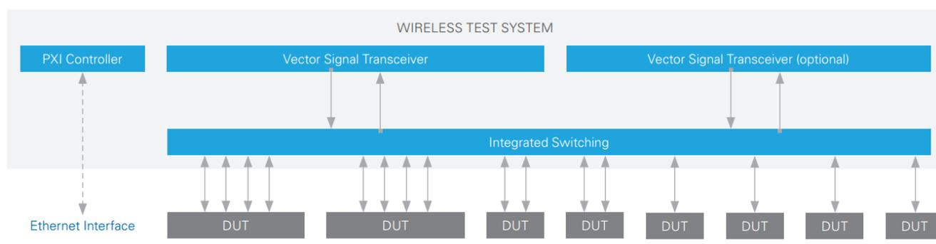
The WTS incorporates an NI vector signal transceiver—a PXI instrument that combines a wideband vector signal generator and analyzer with a powerful FPGA—to help you meet the most challenging wireless test applications.
