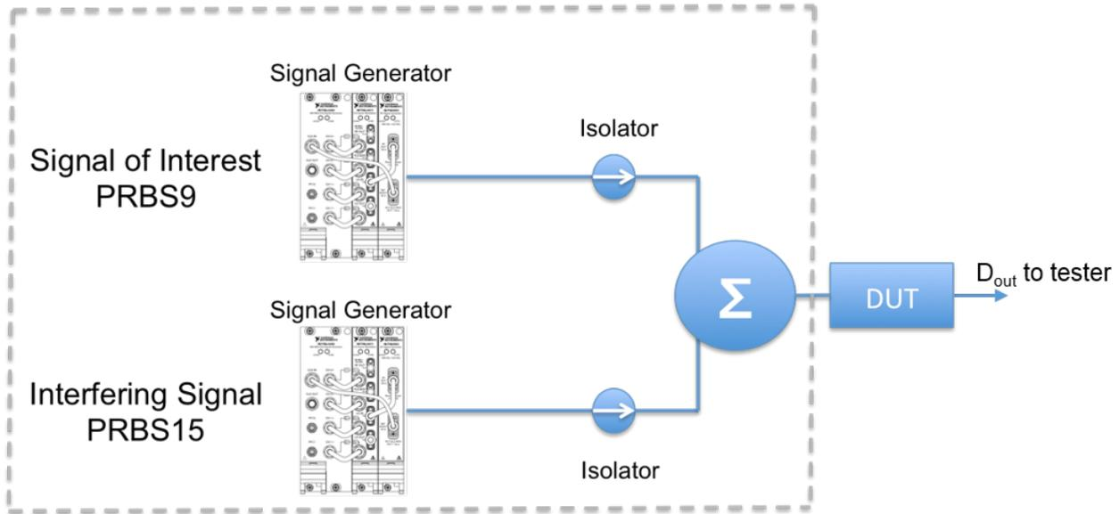
**Figure 53. Blocking Hardware Diagram and Signal Flow**
