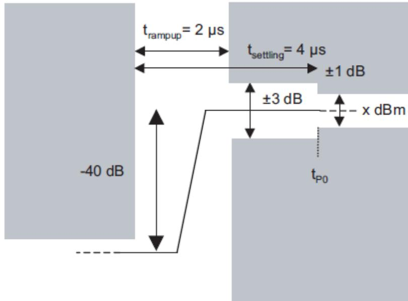
$t_{rampup}$  - time taken for signal generator output power to increase from below -40 dB to with  $\pm 3$  dB of the final output power  $x$  dBm.
