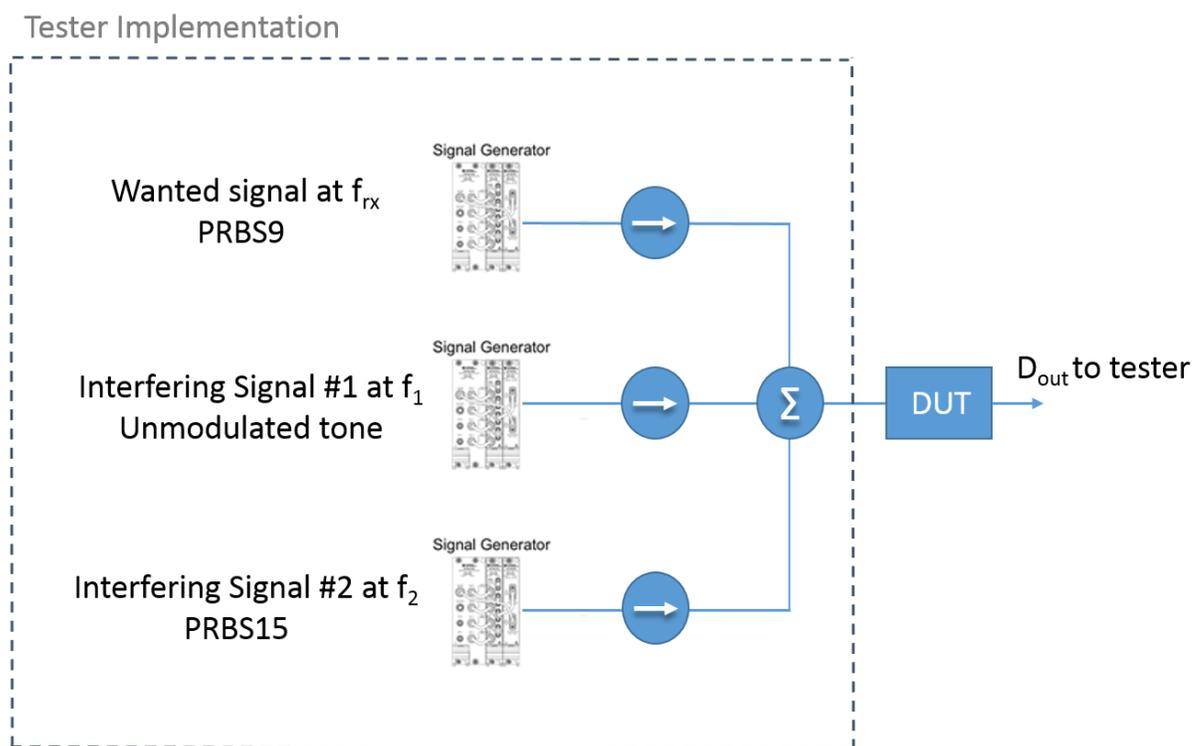
Figure 50. Hardware diagram for intermodulation test
