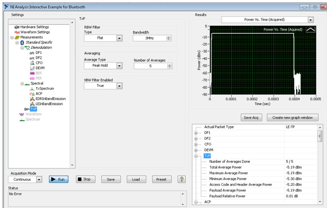
Figure 28. Output Power Measurement (LE packet)
