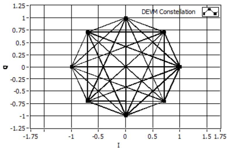
Figure 61 Constellation plot of a 3-DH5 signal.
