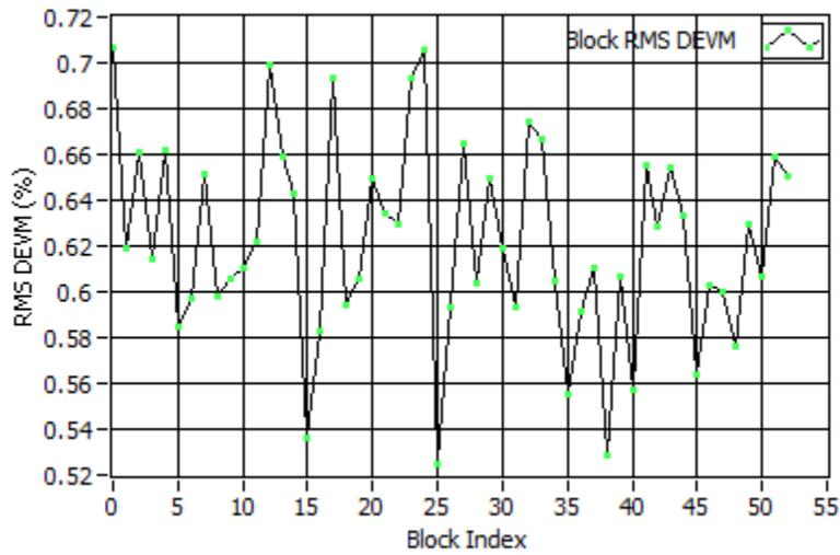
Figure 62 RMS DEVM Measurement Using the NI Bluetooth Measurement Suite
