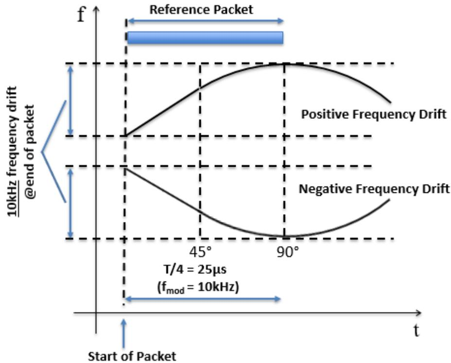
Figure 48 Transmitter Frequency Drift Emulation Principle (EDR)
