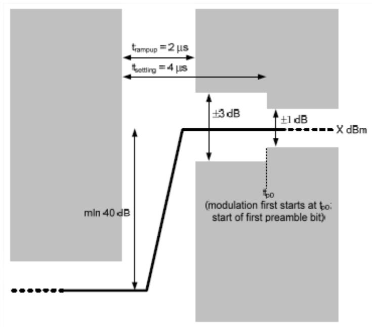
$t_{rampup}$  - time taken for signal generator output power to increase from below -40 dB to with +/- 3 dB of the final output power x dBm.
