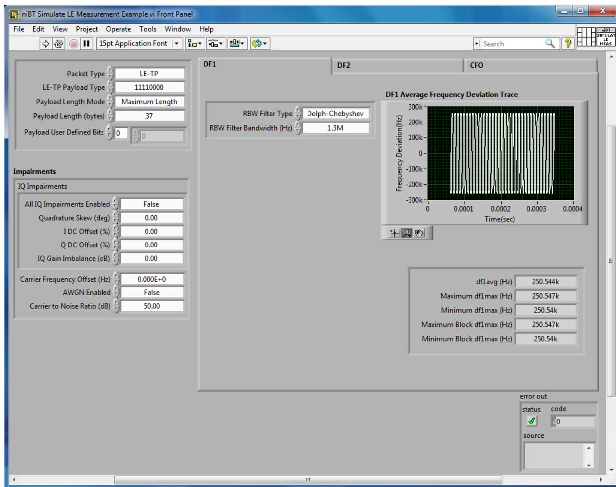
Figure 65 Code to simulate the effects of hardware impairments on the BT signal
