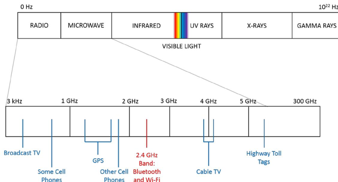
Figure 1 Bluetooth Operating Spectrum
