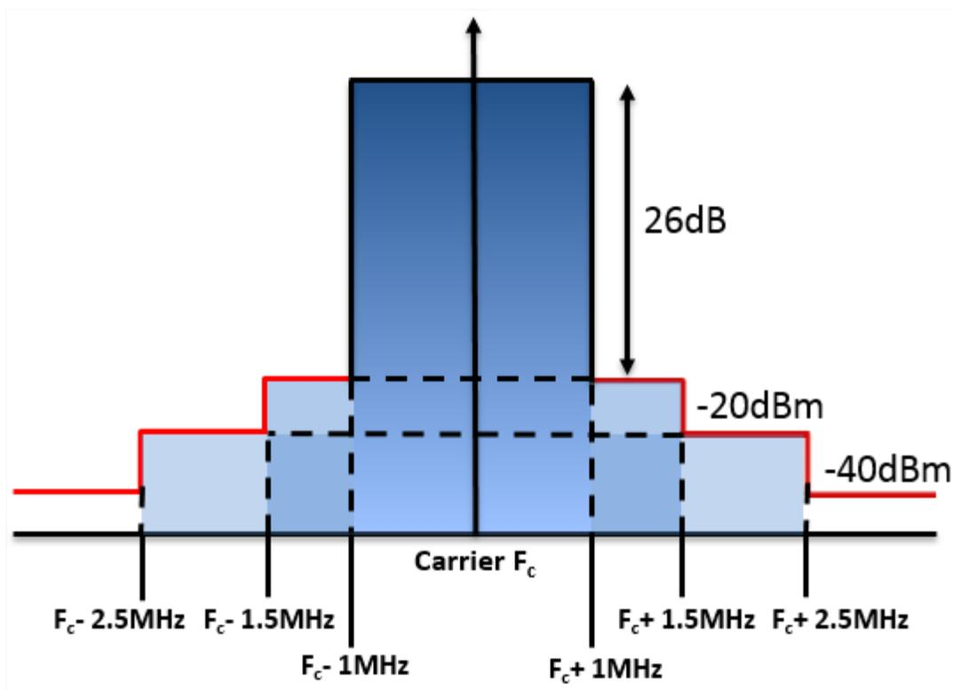
Figure 44. EDR Transmitter Spectral Mask
