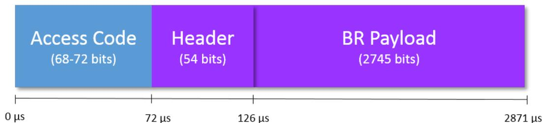
Figure 15. Basic Rate Packet Structure
