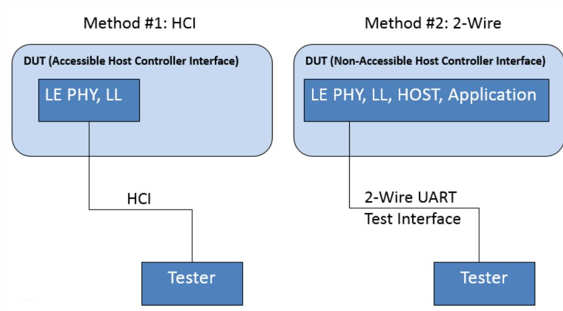
Figure 20. LE Direct Test Mode: Setup Alternatives
