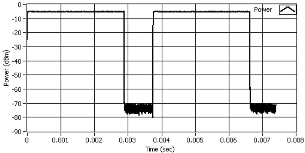
Measurement Interval=7.4ms, Reference Level=-5dBm, Bandwidth=3MHz, RBW Filter Type=Flat; Trigger Level=-25dBm.
