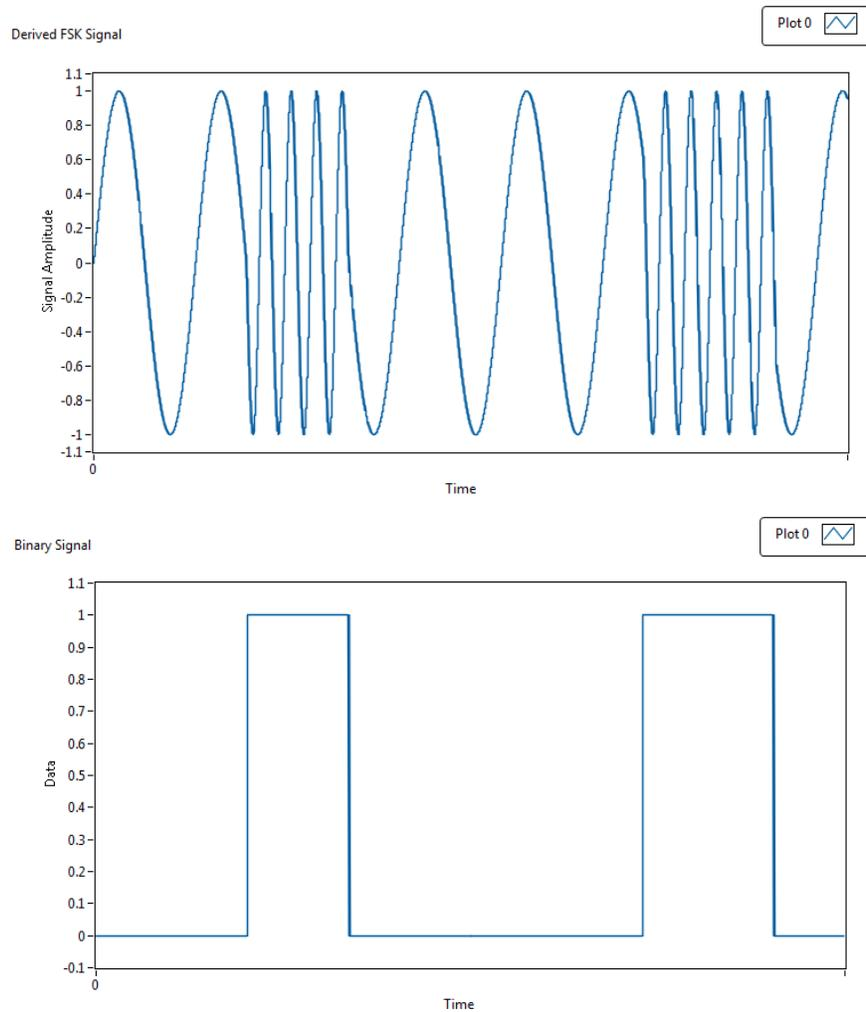
Figure 6. Bits to Waveform Mapping: 2FSK
