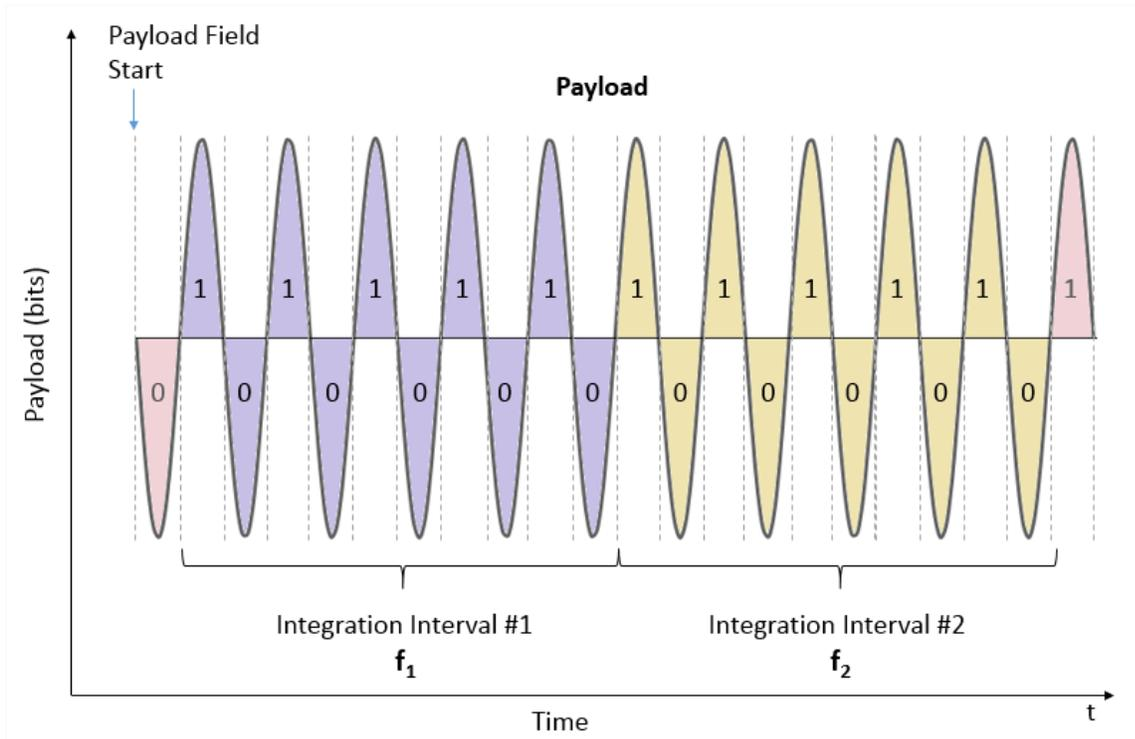
Figure 35. Frequency drift measurement principle
