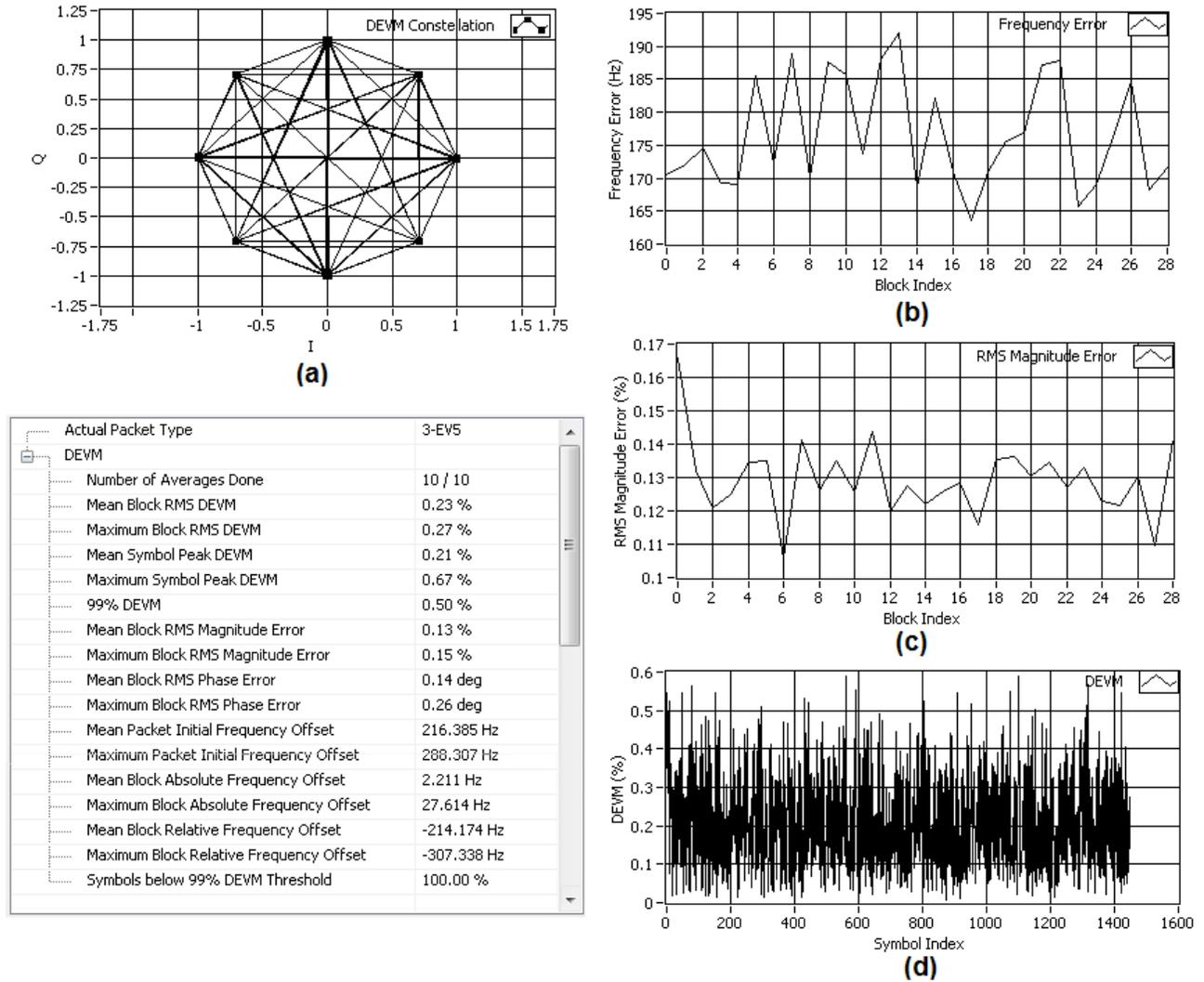
Figure 39. (a) DEVM Constellation for 3-EV5 packet (with 540-byte payload), (b) DEVM Block Frequency Error, (c) DEVM Block RMS Magnitude Error, (d) DEVM Payload Symbol DEVM Trace
