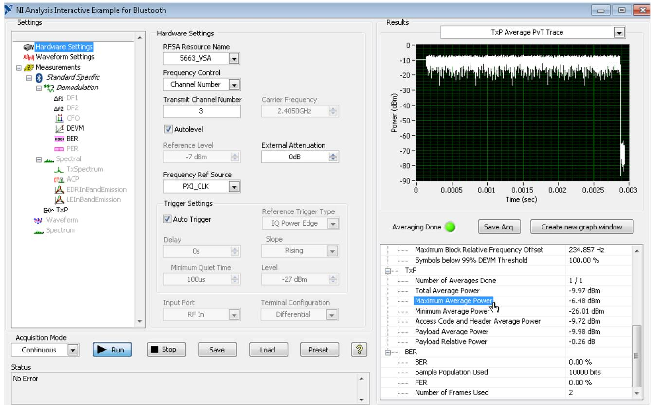
Figure 29 EDR relative transmit power measurement (NI Bluetooth Toolkit)
