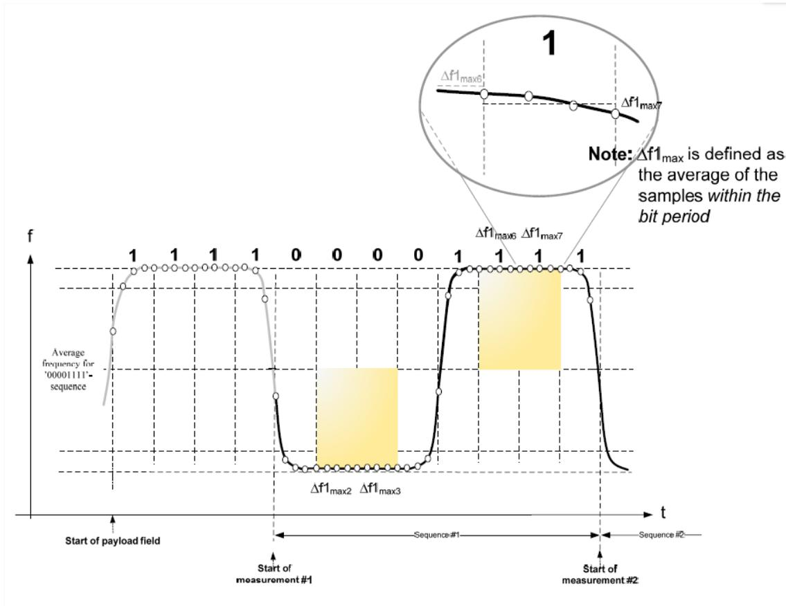
Figure 30. Frequency deviation measurement principle for 11110000-payload sequence [6]
