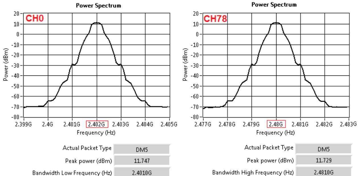
Figure 41. Frequency Range Measurement
