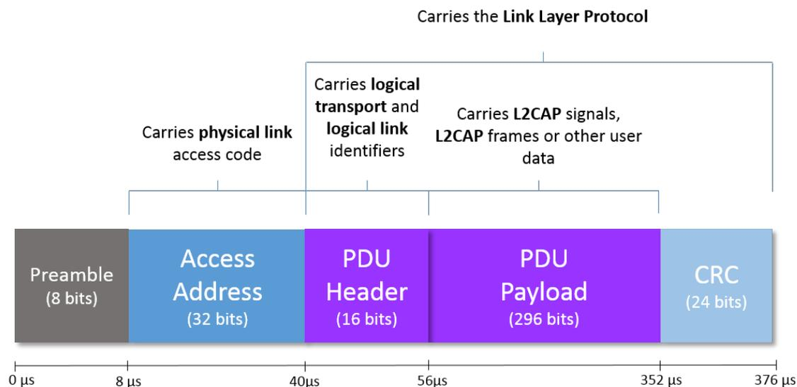
Figure 17 BT LE Packet Structure (1 Mbps)
