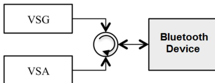
Figure 25. Typical test setup for a Bluetooth device
