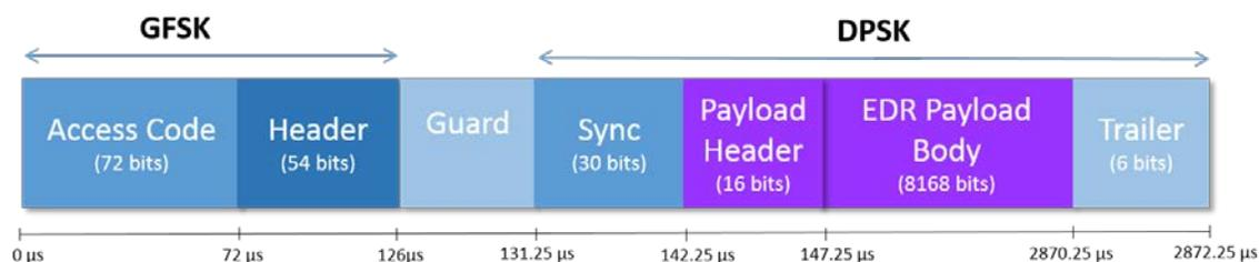
Figure 16a. EDR Packet Structure (3-DH5 with full max payload and 5.25 μs guard band)
