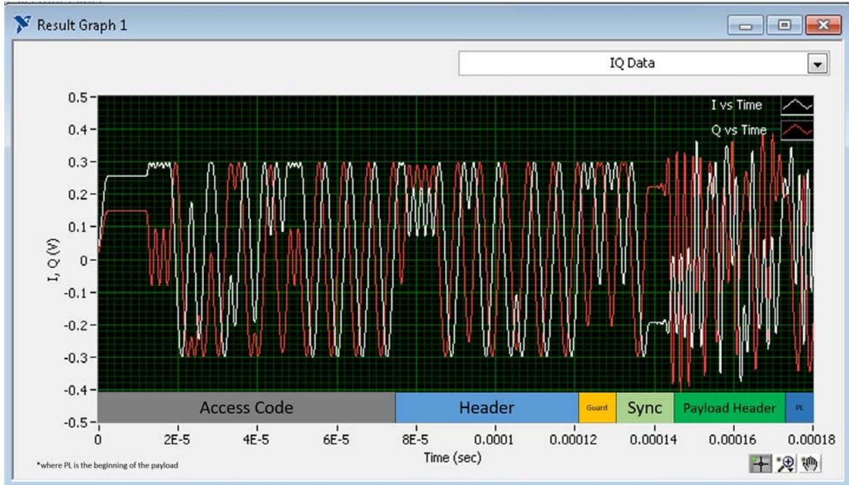
**Figure 17b. 3-DH5 Packet Structure and Timing**
