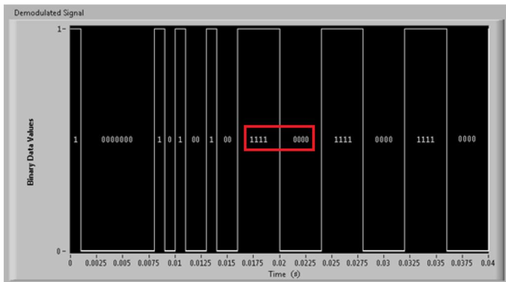
Figure 24. Demodulated LE packet with 11110000 payload pattern (NI Bluetooth Analysis Toolkit)
