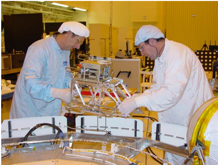
IVSR being installed on Cruise Stage
