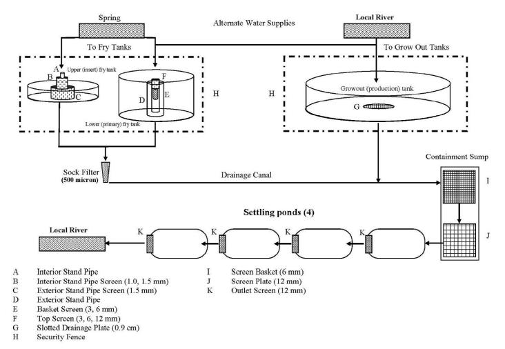
Figure 9. Schematic Summary of Containment Measures at the Grow-Out Facility
