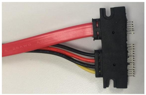
\* Pin 1 (ground) broken by accident, no impact due to redundant Pin 4 and Pin 7
