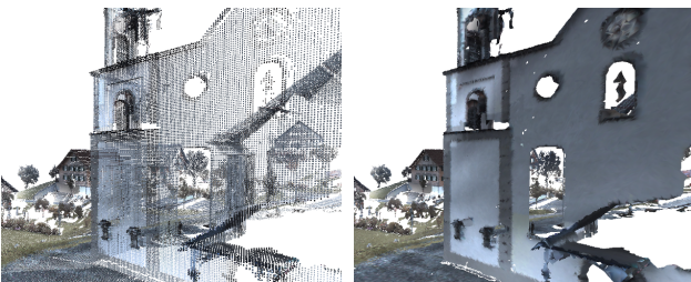
Figure 3: Point cloud (left) and mesh (right) seen from the same point of view: dense representations help understanding the scene.
