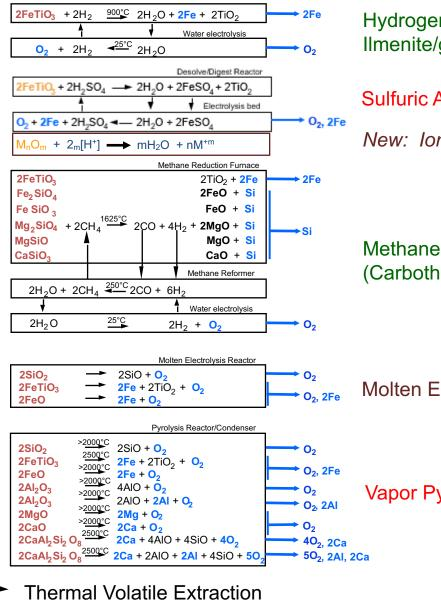
Hydrogen Reduction of Ilmenite/glass Process
