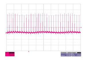
Figure 29. Ripple at +6-V Output with V<sub>IN</sub> = 1200 V DC and Full Load
