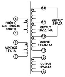
Figure 18. Transformer Pinout
