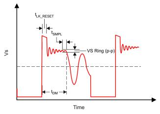
Figure 7. Aux Waveform — Sampling
