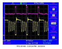
Figure 22. Upper FET Voltage at 1200-V Input, 50-W Output (CH3:  $V_{gs}$  and CH1:  $V_{ds}$ )
