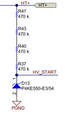
Figure 16. Start-Up Circuit
