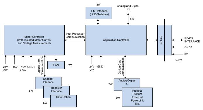
Figure 2. Drive Control Architecture with Typical Power Consumption
