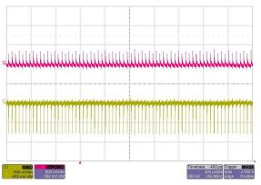
Figure 27. Ripple at  $\pm$ 16–V Output with V<sub>IN</sub> = 1200 V DC and Full Load (CH2: +16 V, CH1: -16 V)
