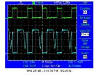
Figure 19. Lower FET Voltage at 400-V Input, 50-W Output (CH4:  $V_{qs}$  and CH2:  $V_{ds}$ )
