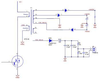
Figure 17. DC Link Voltage Measurement
