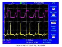
Figure 20. Upper FET Voltage at 400-V Input, 50-W Output (CH3:  $V_{ds}$  and CH1:  $V_{ds}$ )
