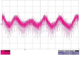
Figure 25. Ripple at 24-V Output with  $V_{IN}$  = 1200 V DC and Full Load
