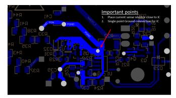
Figure 44. Layout Diagram One
