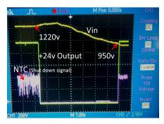
Figure 42. DC Link Voltage Measurement with Full Load
