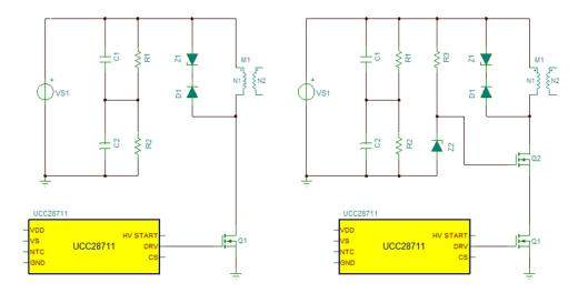
Figure 3. Flyback Controller with Single and Dual MOSFET Switch
