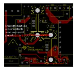
Figure 46. Layout Diagram Three
