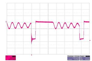
Figure 23. 24-V Output Diode Voltage Stress with  $V_{IN}$  = 1200 V DC and 50-W Output
