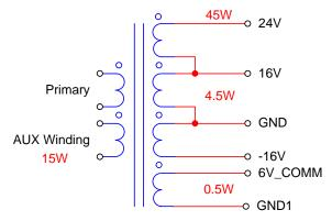
Figure 5. Transformer Configuration
