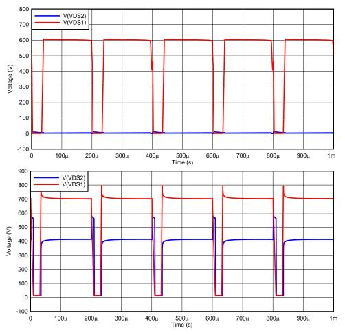
Figure 4.  $V_{DS}$  Voltage of MOSFETs During Low  $V_{IN}$  and High  $V_{IN}$
