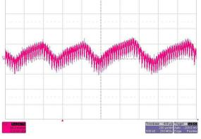
Figure 24. Ripple at 24-V Output with V<sub>IN</sub> = 400 V DC and Full Load
