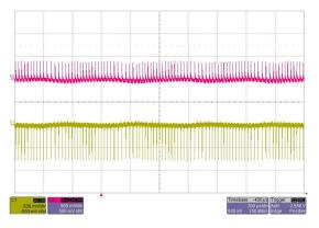
Figure 26. Ripple at ±16-V Output with  $V_{IN}$  = 400 V DC and Full Load (CH2: +16 V, CH1: -16 V)
